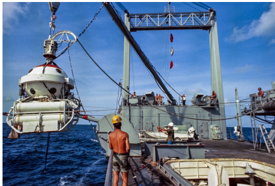
The Personnel Transfer Capsule suspended outboard of YDT-16, the deck gantry and support crew visible aft. The capsule carried divers between the deck decompression chambers and working depth.
