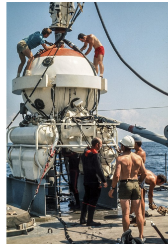
Crew working atop the Personnel Transfer Capsule on deck between dives, the ballast cylinders and mating hatch clearly visible.
