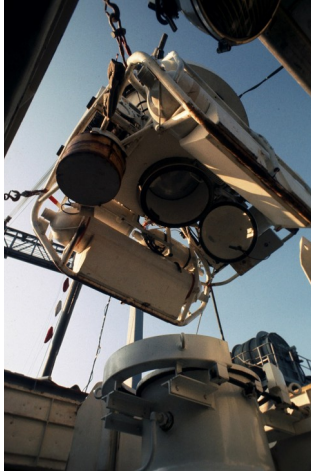
Looking up at the Personnel Transfer Capsule from the deck of YDT-16, its viewports and lower mating flange visible, with the deck chamber trunk below.
