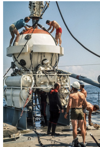
Crew working atop the capsule on deck between dives, the ballast cylinders and mating hatch clearly visible.
