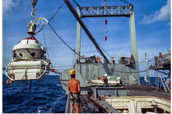
The capsule suspended outboard, the deck gantry and support crew visible aft. It carried divers between the deck decompression chambers and working depth.
